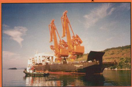
In February 1995, two ship unloaders were safely delivered to the refurbished Guacolda pier in Huasco, Chile. The unloaders were shipped fully erected by Trinav Shipping (Barbados) Ltd., using the Russian heavy lift ship Stakhanovets Ermolenko. Argonautics Marine Engineering of Sausalito, Calif., provided all the engineering and supervision required for the safe load-out, seafastening, transportation and offloading of the unloaders.
